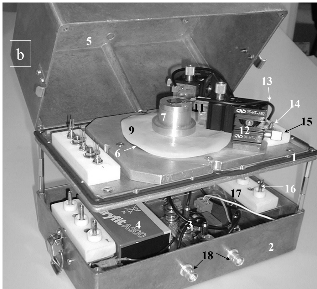
Fig. 1. Schematic view (a) and photograph (b) of the probe system for wafer level noise measurements.
